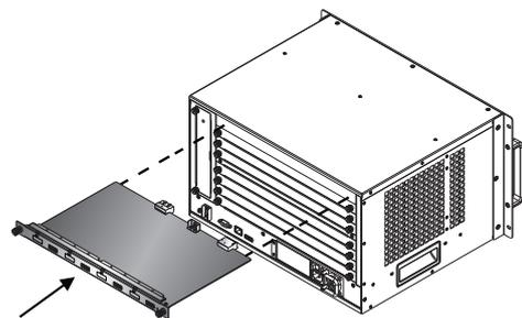
4. Tighten the two screws on the VM7104 board to fasten it to the Modular Matrix Switch, until it's secured to the unit
