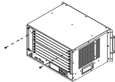
3. Slide the VM7104 board into the open slot on the VM1600 until it secures in place.
